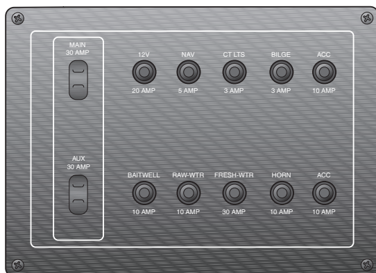
TYPICAL BREAKER / FUSE PANEL
