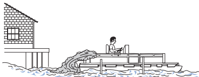
Blockage of boat exhaust by obstruction
