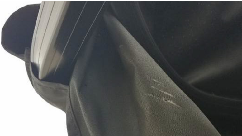
Damage due to pivoting bows
